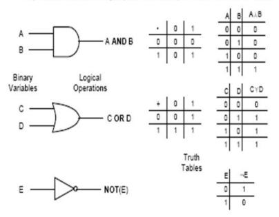
Considering the truth tables, draw a simple circuit that would be logically equivalent to  $p \rightarrow q$
